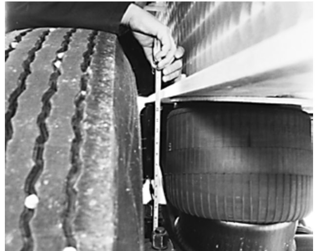
Figure 30: Measuring ride height with tape measure
