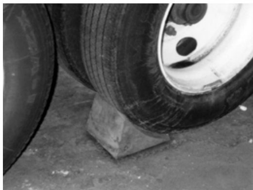
Figure 26: Chock trailer wheel
