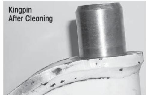
2. Inspect the kingpin for wear or damage. Use a micrometer and measure the upper and lower kingpin in two locations. Positions must be 90° opposed from each other. If the kingpin has less than 1.802" diameter, replacement of the axle is necessary, see Figures 9-39 through 9-42.
