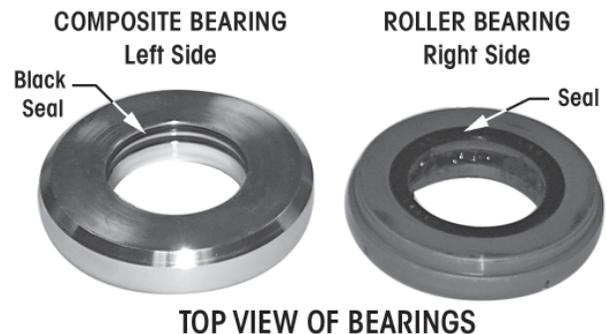
1. Install the thrust bearing on the lower kingpin with the seal facing up toward axle (the black seal will designate the top side), see Figure 9-60.
