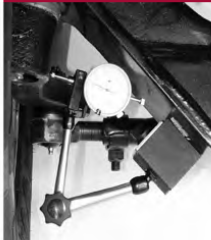
CHECK LOWER KINGPIN BUSHING
