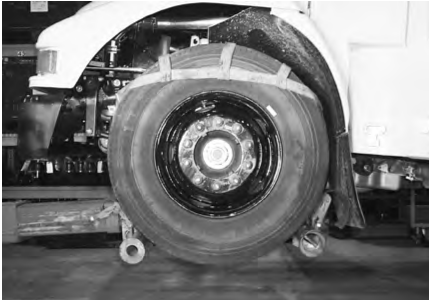
FIGURE 6-1 Wheel lift method
