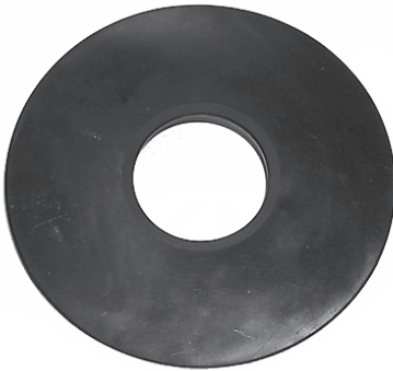
Normal bushing tube spacer in serviceable condition.
