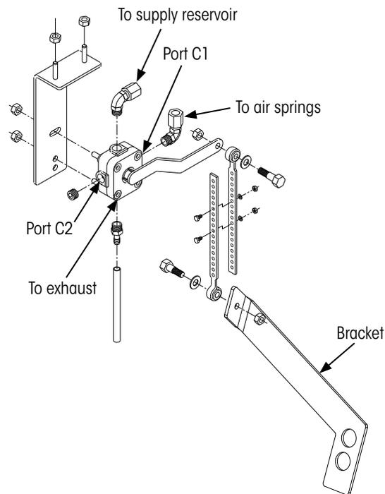
Figure 7: HCV assembly for VANTRAAX® HKANT suspensions
