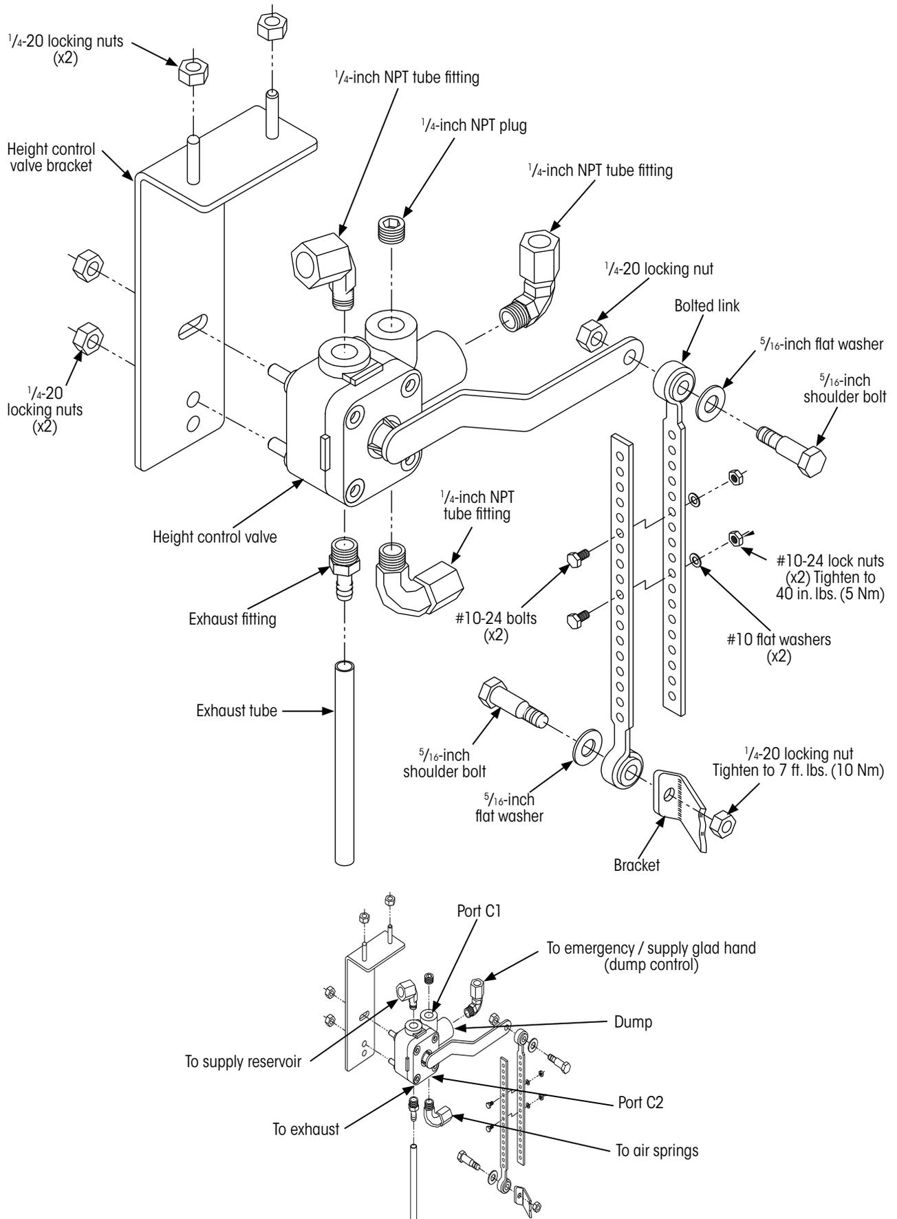
Figure 8: Integral dump HCV assembly for VANTRAAAX® HKANT suspensions
