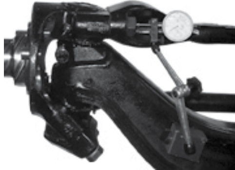
CHECKING UPPER KINGPIN BUSHING
