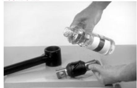
2. Lubricate the inner diameter of the torque rod end hub and the new rubber bushing (see Figure 8-22) with P-80 Lubricant (refer to Parts List Section in this publication) or light Naphthenic Base Oil, such as 60 SUS at 100°F.
