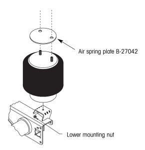
80-100 ft. lbs. (108-136N•m). If the entire air spring was replaced, tighten the lower mounting nut to a torque of 40-50 ft. lbs. (54-68N•m).
