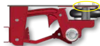
Primary (airbag) bump stop engages
