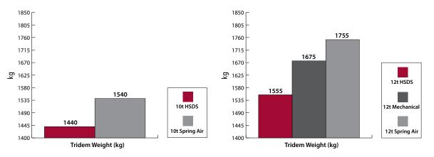
Weight includes the suspension system and related components. Above data are based upon internal testing and / or published specifications.
