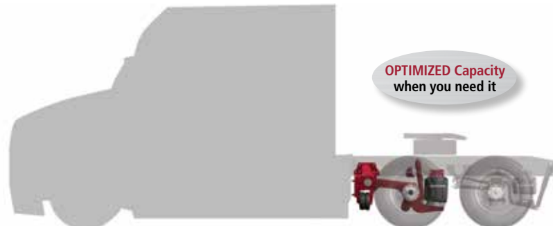
Axle lowered for 6×2 configuration — The OPTIMAAX system senses higher load conditions and lowers the non-drive axle
