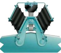
and stability throughout the empty and loaded condition. The rubber portions of the bolster spring is bonded to steel
