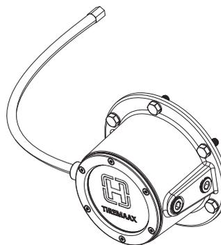
Figure 27: Super-single tire hose to hubcap connection
