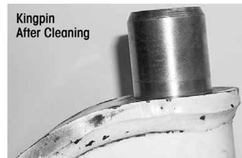
2. Inspect the kingpin for wear or damage. Use a micrometer, measure the upper and lower kingpin in two locations. Positions must be 90 degrees (perpendicular) from each other, see Figures 8-6 through 8-9.
