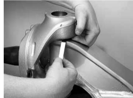
9. Insert feeler gauges between the upper kingpin connection and the top of the axle. Check the clearance between the upper kingpin connection and the top of the axle (See Figure 8-27).
