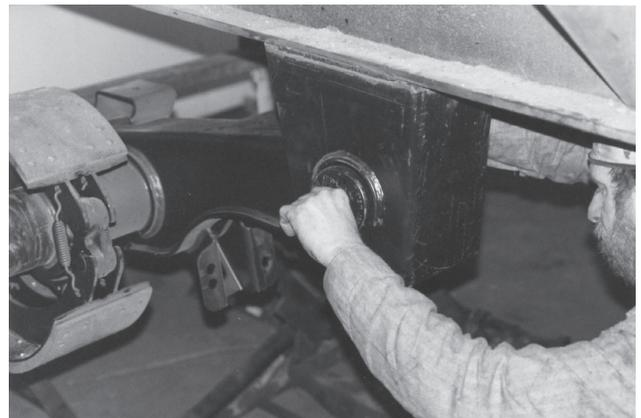
Figure 9: Installing new pivot connection hardware
