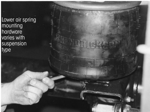
Lower air spring mounting hardware varies with suspension type
