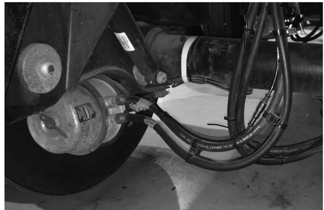
Figure 3: Brake chamber
