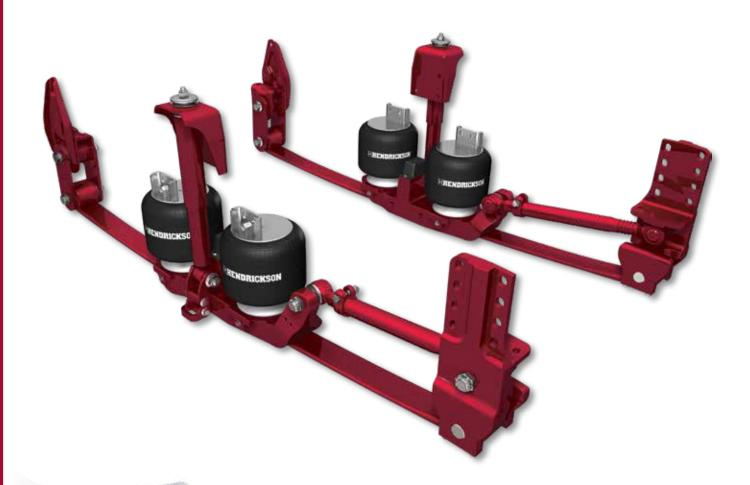
The Front Air Assist suspension system offers premium ride comfort comparable to that of a full air suspension in a compact package. Hendrickson's system features a high wheel cut with tighter turning radius with no spring wind-up or castor change providing excellent steering and directional stability. An extra-long travel suspension with raise and lower capability provides superior vehicle protection and flexibility in cargo handling.
