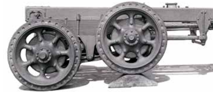
Hendrickson's invention of the first tandem "walking beam" suspension established the company as an innovator.
