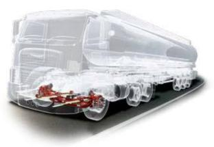
Hendrickson's STEERTEK NXT front steer axle and integrated suspension are optimised to deliver maximum performance as a complete system solution. The fabricated STEERTEK NXT design integrates lightweight axle durability with advanced composite spring suspension technology, saving weight compared to traditional I-beam axle and multi-leaf spring systems.
