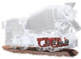
Rated up to 11.5t (single) / 23t (tandem), PRIMAAX® EX air suspension provides optimal ride performance and excellent articulation. Unique parallelogram suspension geometry, to significantly control drive / brake torque, with cast support beams and square cross brace provides a solid connection and forms a rigid torsion and stabiliser system providing optimal roll stability and directional control.
