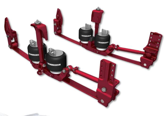
The FRONT AIR ASSIST suspension system offers premium ride comfort comparable to a full air suspension in a compact package. Hendrickson's system features a high wheel cut with a tighter turning radius and no spring wind-up or castor change providing excellent steering and directional stability. An extra-long travel suspension with raise and lower capability provides superior vehicle protection and flexibility in cargo handling.
