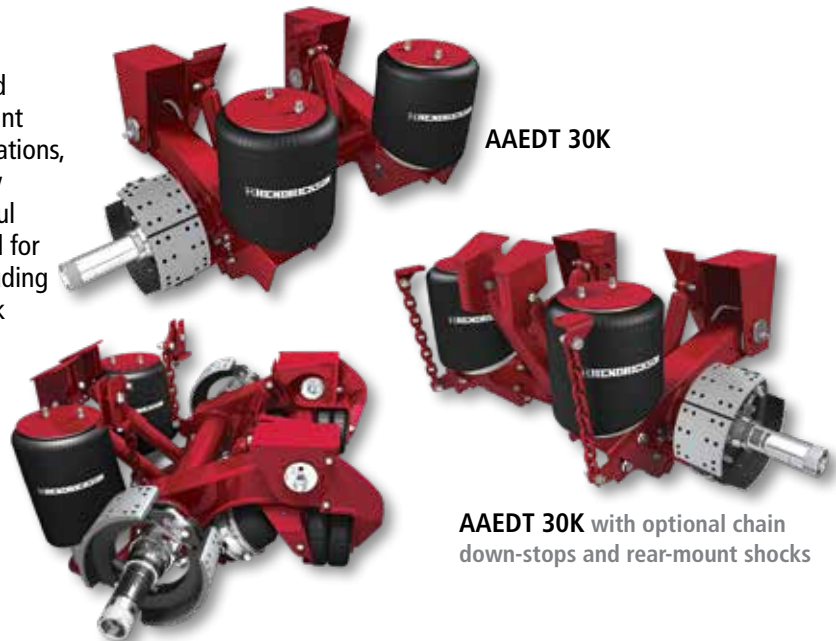
AAEDL 30K with optional chain down-stops, rear-mount shocks and UBL™ UNDER BEAM LIFT™
